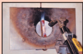
Fire test of protective sleeveings
